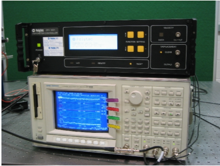
Figure B.4. Polytec OFV-3001 Controller(top) and Onisoki FFT Analyzer with Signal Generator(bottom).
